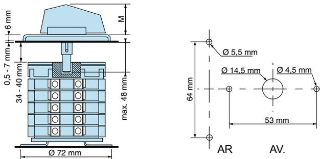
Panel cut-out where AV attachment is used with M6 or M7 lockable handles.
