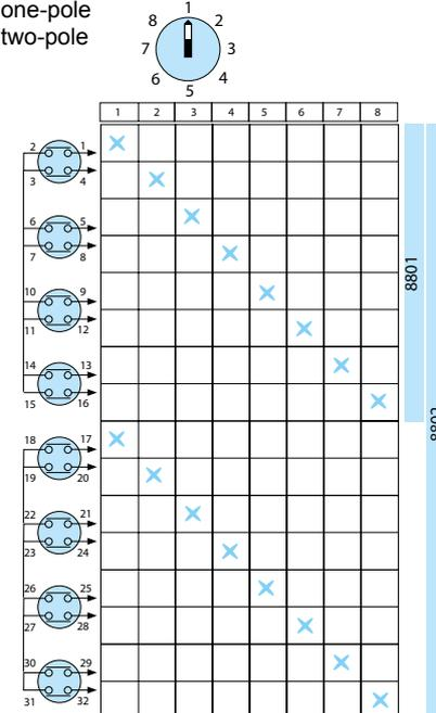
3 positions inverter (with intermediate stop)
